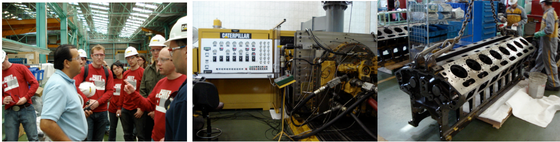
From left to right: Plant Manager gives a facility tour to UBC students. Caterpillar's in house dynamometer can test engine and transmission performance. An engine block being refurbished.
