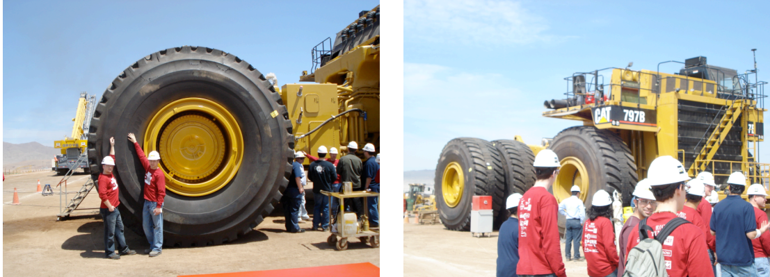
Above: Construction of a Caterpillar 797B Haul Truck. Truck to be delivered to the Escondida Mine Site.
